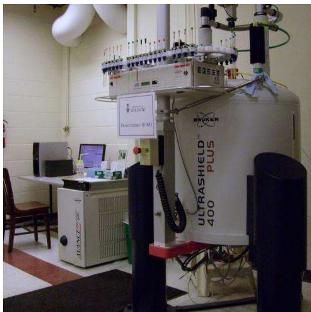
The NMR spectrometer used in TCG Lifesciences, Kolkata, as we observed, was Buckner Ultrashield 400 with capacity upto 400 MHz.
